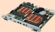
Dual/single Intel® Xeon® E5-2600 Series Processors CPU ATCA blade with 40GbE fabric ports
