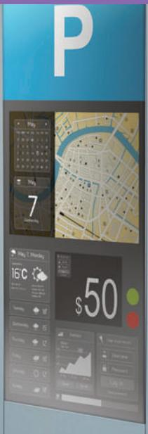
Smart Parking Systems include vacant parking space detection with direction indication, number of available parking spaces, payment systems, and advertising. Advantech offered a reliable embedded solution to meet all these functions for this self-service kiosk application ranging from embedded computing platform, touch display, SATA SSD, and WISE-PaaS/RMM remote management software.
