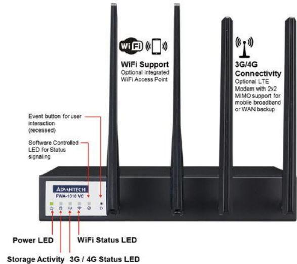
In contrast to externally attached wireless dongles, it also secures the SIM card within the unit to avoid unwanted removal which would result in end customer service interruptions and increased support efforts for the service provider.
