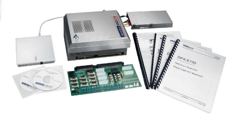
The kits are based on a DPX® mainboard, and includes all the other necessary items to set up an evaluation and development station.
