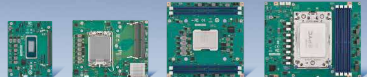
Client Size A Client Size C Server Size D Server Size E
