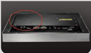
HDD door design for easy maintenance
