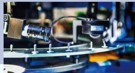
Multi-Angle Inspection for Manufacturing Defects
